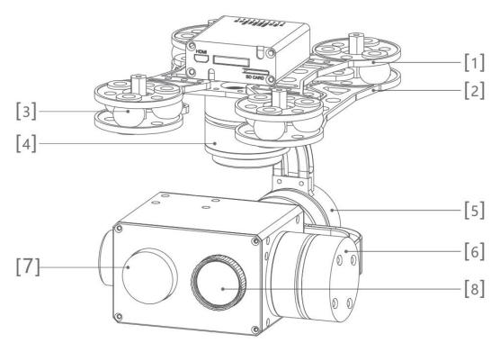
[1]Upper damper board[3]Rubber damper[5]Roll axis motor[7]Thermal camera
