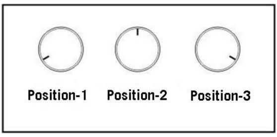
Rotate knob to position-3:low speed lock mode. The gimbal will move at the lowest speed when controlling YAW and PITCH, and gimbal YAW axis will not follow drone flight direction.
