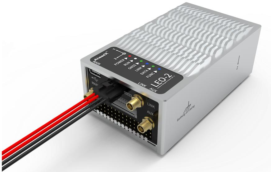
Then connect 7-53v power supply to the device, the POW led will keep being on, and the RUN led will flash, proving that the device is working, as shown below:
