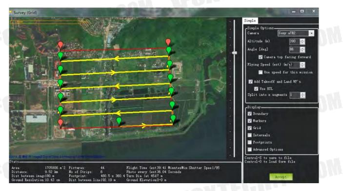
If you accept these parameters, please click accept, the mission plannaer will generate a series of waypoints covering the designated area, including the take-off point and the landing point. Call DO\_SET\_ CAM\_TRIGG\_DIST command to set the distance of the camera shutter command, and finally call DO\_SET\_ CAM\_TRIGG\_DIST again to set the parameter back to 0 and stop taking pictures; note that the parameters of two call are different.
