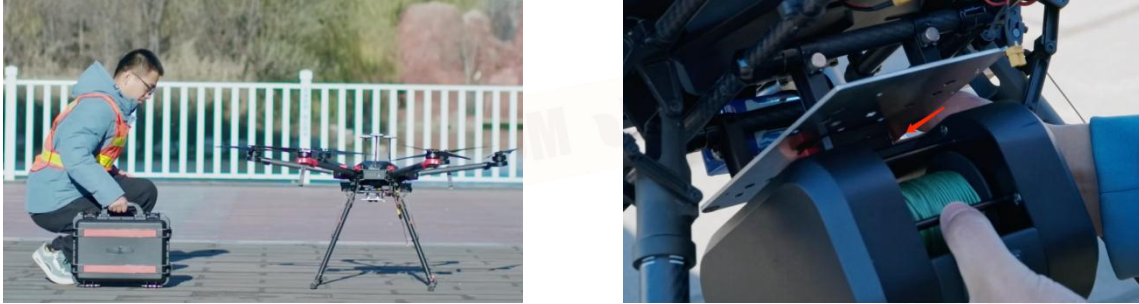
FIG 5-3-1 The installation of the winch body on the aircraft platform
