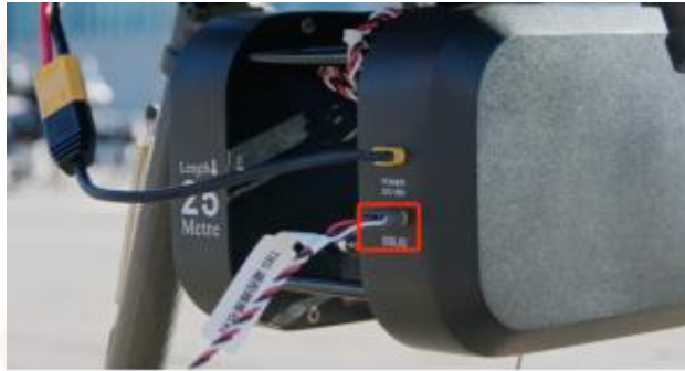
FIG 5-4-2 The SBUS cable into the winch SBUS
