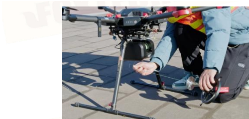
FIG 7-1-5 Lower the cable to a sufficient length
