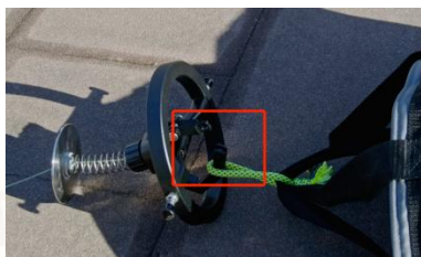
FIG 7-1-7 Hang it into the groove
