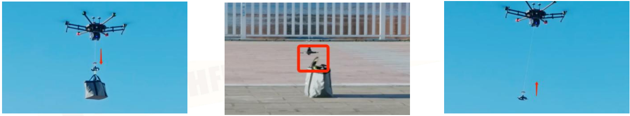
FIG 8-1-5 unload the cargo (mechanical release without the safety pin)
