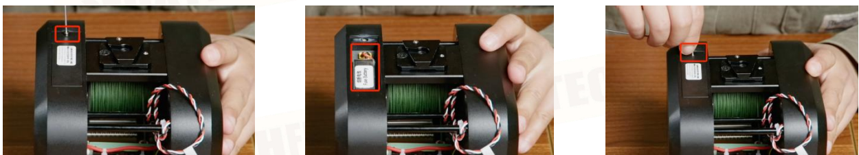
FIG 5-2-1 Fuse battery installation
