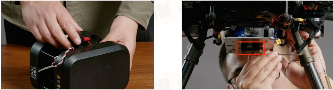
FIG 5-1-1 Show the quick-release mounting installation on drone
