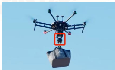
FIG 7-2-6 winch rises to the limiter
