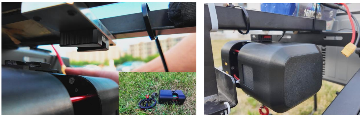
FIG 5-2-1 The installation of the winch body on the aircraft platform
