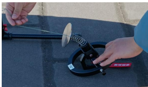
FIG 5-3-3 Ensure that the rope is not tangled & the unhooker is reset
