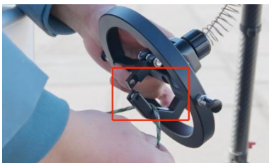
FIG 7-1-3 Hang it into the groove
