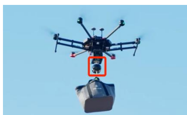
FIG 7-2-6 winch rises to the limiter
