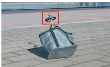
FIG 7-1-8 confirm to lift the cargo
