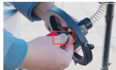
FIG 7-1-4 Insert the safety pin
