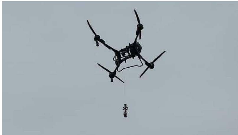
FIG 3-1-1 UAV platform equipped with 15KG winch for drone system
