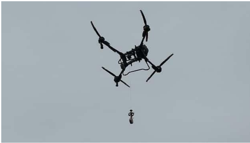
FIG 3-1-1 UAV platform equipped with 25KG winch for drone system
