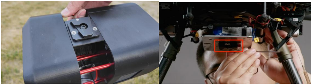
FIG 5-1-1 Show the quick-release mounting installation on drone
