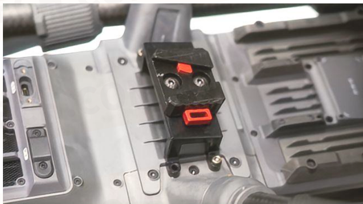
FIG 5-1-1 Installing the Quick-Release Mount on the UAV Platform (For Reference Only)
