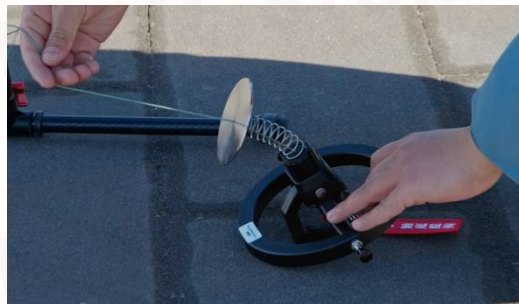
FIG 5-6-1 Checking for Cable Entanglement and Resetting the Release Hook
