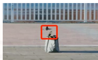
FIG 8-1-5 Cargo Unloading (Mechanical Release Hook Without Safety Pin)
