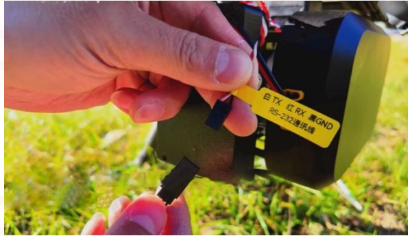
FIG 5-3-3 PSDK Adapter Module Communication Cable Installation
