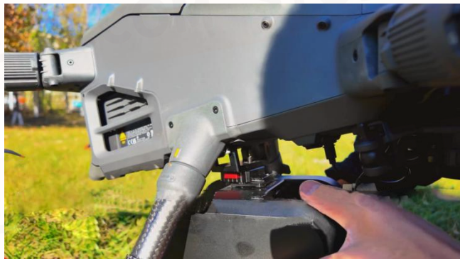
FIG 5-4-1 Installing the Winch Main Unit on the UAV Platform
