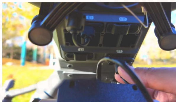
FIG 5-4-2 Connecting the PSDK Adapter Module to DJI E-Port V2
