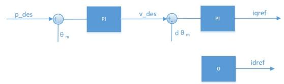
p\_des is the target position for control, and v\_des limits the maximum absolute speed during motion.
