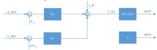
Derived from the MIT mode, various control modes can be implemented. For example:
