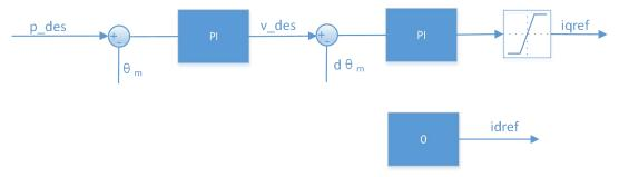
A current command saturation stage is added after the speed loop output, which limits the current loop command within a specified range.
