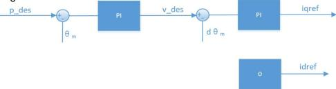
p\_des is the target position for control, and v\_des limits the maximum absolute speed during motion.
