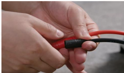
FIG 5-5-3 Disconnect Power Supply
