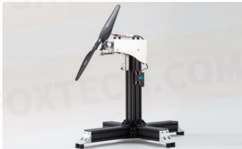
FIG 3-1-1 LY-30KGF thrust stand
