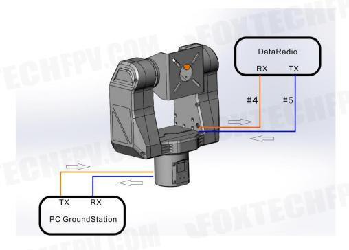
Connect your GroundStation to the DataRadio via the slipring of the Crossbow AAT
