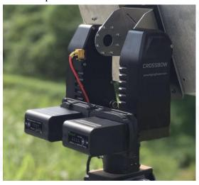
2. The antenna has to be mounted on the Archer AAT with the use of a special bracket.In order to prevent tampering with the normal operation of the compass built into the Archer AAT it is recommended to avoid using antennas made with ferromagnetic materials. Wherever possible, use non-magnetic stainless steel bolts, aluminum and other non-magnetic materials.
