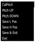
Use this function to calibrate the pitch sub-system of your tracker.
