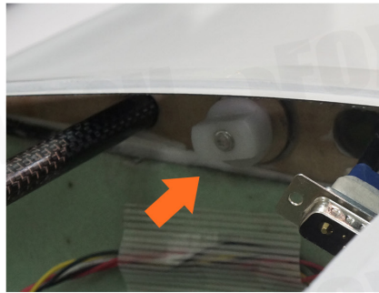
5. Tighten the four screws for the aileron inside the body. (Two screws are in the central section and two are in the front section.)
