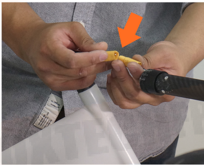
7. Connect the servo cable.
