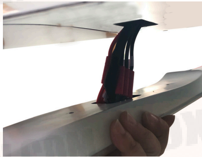
5. Connect the cables in the arm and then fix the arm.
