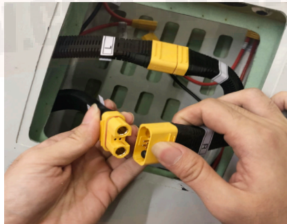
2. Connect the Main Cable. (including ESC signal cable, ESC power cable, servo signal cable)
